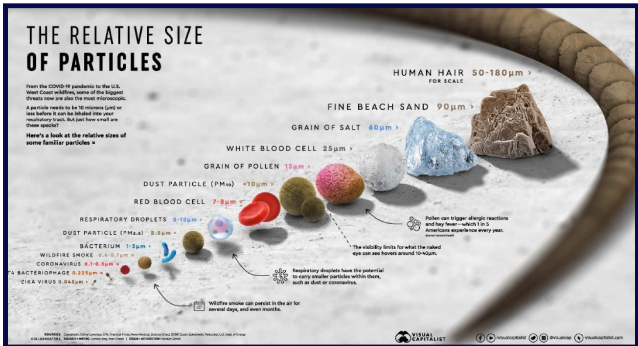
Figure 4 legend. Mechanical filtration in HVAC filters is dependent upon the exclusion by the filter material of particles of various sizes. The SARS CoV 2 virus as an aerosol has an approximate diameter of 0.3 µm. Viruses are among the smallest particles that can be excluded by filters
